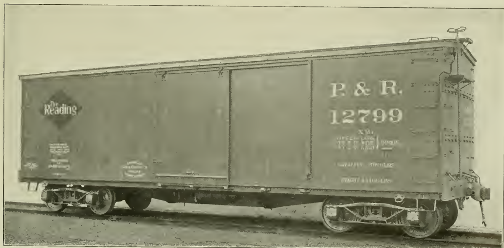
Steel Underframe Box Car with Reinforced Ends; Philadelphia and Reading.
